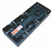
AVFS 3080 Floor Spring - Single Crock, (Door Weight 80kg) Max. Door Width 850mm, Cover Plate Finish - SSS
